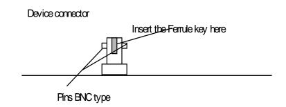
To install the connector, Side the ferrule key gently into the above key. Then, turning, insert the two BNC pins into The appropriate slots on the ST connector.
