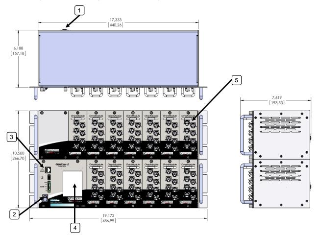
1) 20-28 Volt DC power connector: You must use a DC power supply. It is highly recommended to use the power supply module that is shipped with your OFX2 chassis.
