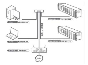
b) You connect the OmniFlex-2 through a dedicated Ethernet interface and cable, using a "private" network arrangement. Furthermore, to keep your organization network operational at the same time, you will need an additional Ethernet interface / adapter, such as a USB to Ethernet device (this can be purchased for a nominal fee at any computer store). This has the advantage of keeping the OFX2 isolated from all outside networks and thus will provide the best security scheme.
